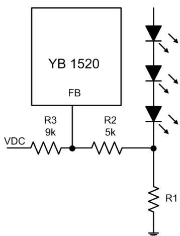
Figure 4: Dimming Control Using a DC Voltage
