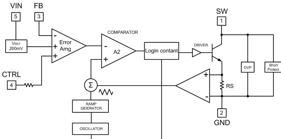
Figure 3: YB1520 Block Diagram
