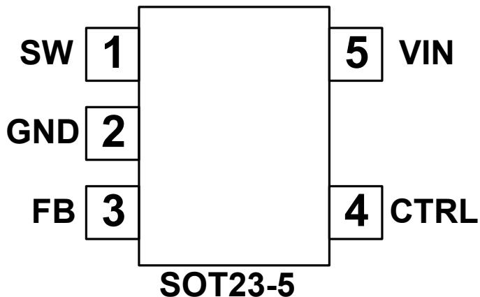
Figure 2: Pin Configuration
