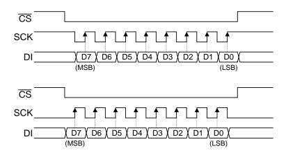
• SCK falling Edge Operation (DIPH pin is at "H" level)
