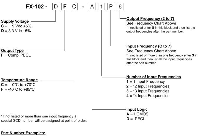
FX-102-DFC-D1P6 \*FX-102-DFF-A4S6, S = 8 kHz, 1.544 MHz, 2.048 MHz, 19.44 MHz \*FX-102-DFC-D16S, S = 166.6286 MHz
