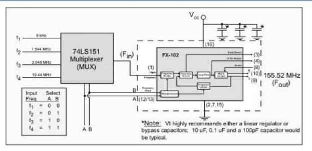
All components outside the dotted line box are user supplied components. This is just one possible configuration of the FX-102. For additional information about your specific needs, please contact our factory.
