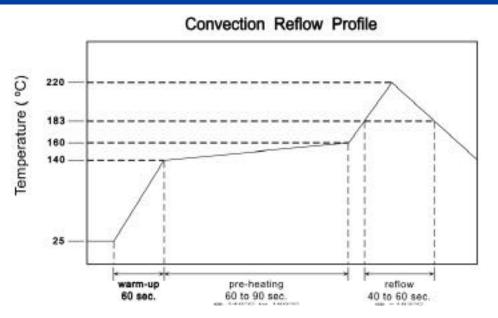
**NOTE:** The FX-100 series should not be subjected to a wash process that will immerse it in solvents. NO CLEAN is the recommended procedure. The FX-100 series has been designed for pick and place reflow soldering. The suggested reflow profile is shown above. The FX-100 series may be reflowed once, and should not be reflowed in the inverted position.
