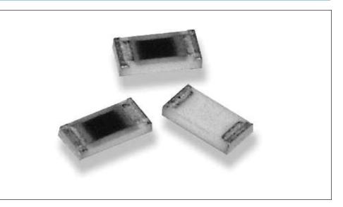
Precious metal terminations are screen printed onto a ceramic base and fired. The resistive element is screen printed and fired and the passivation layer added. Each resistor is trimmed to tolerance by sand blasting. The prescribed tile is broken into strips, the end plating is fired on and the strips broken into individual components. Final termination is made by electroplating.
