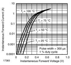
Figure 5. Typical Instantaneous Forward Characteristics - SL03
