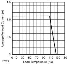
Figure 1. Forward Current Derating Curve
