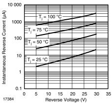
Figure 6. Typical Reverse Current Characteristics - SL03
