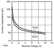
Figure 2. Typical Junction Capacitance
