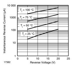
Figure 4. Typical Reverse Current Characteristics - SL02
