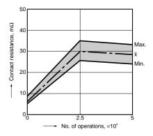
5-(3). Electrical life test (UL lamp load test TV-4)
