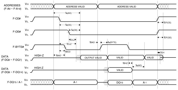
When F-BYTE#=VIH, F-CE#=F-OE#=VIL, DQ15/A-1 is output status. At this time, input signal must not be applied.
