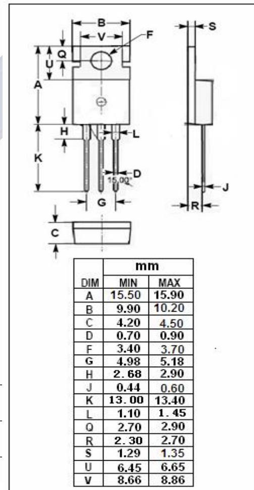
**isc N-Channel MOSFET Transistor**
