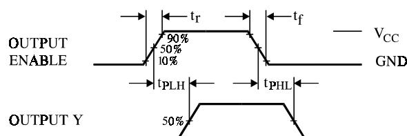
Figure 3. Switching Waveforms
