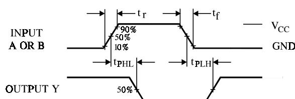
Figure 1. Switching Waveforms
