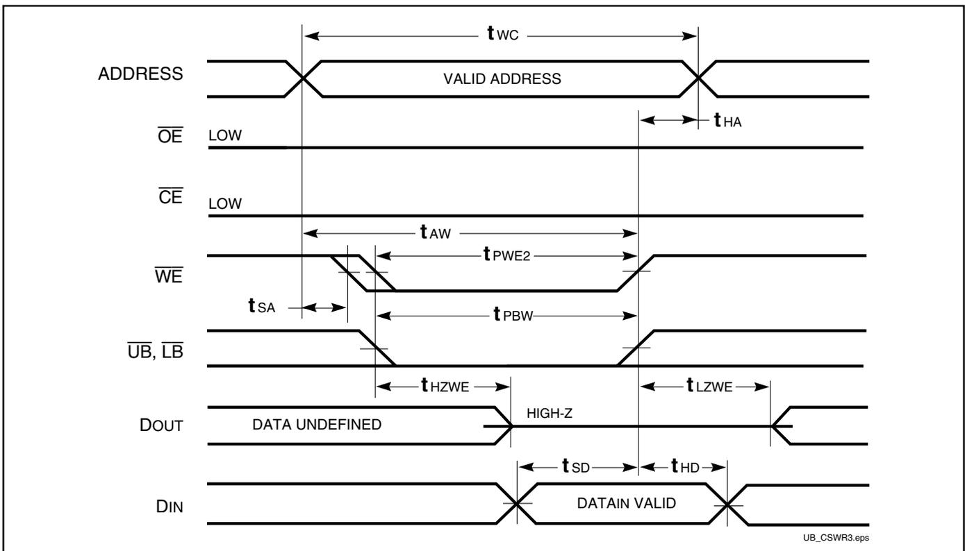
WRITE CYCLE NO. 4 ( $\overline{UB}/\overline{LB}$  Controlled)
