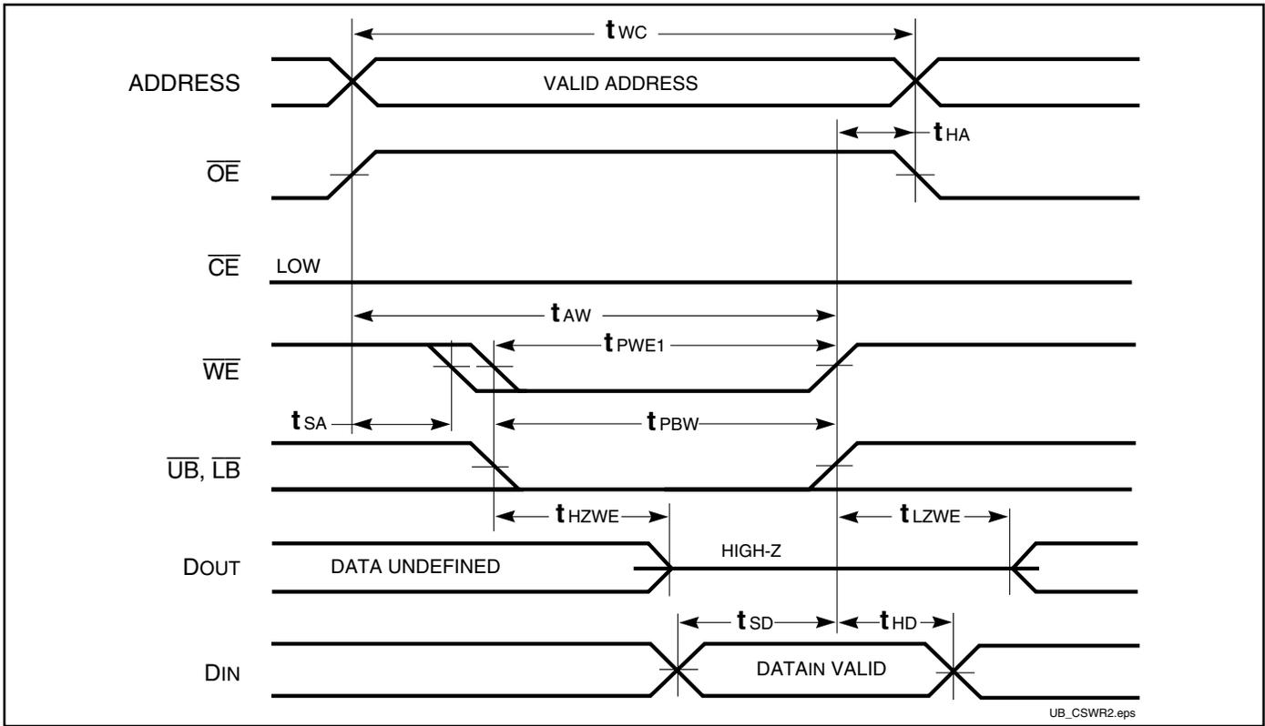
**WRITE CYCLE NO. 3** ( $\overline{WE}$  Controlled:  $\overline{OE}$  is LOW During Write Cycle)
