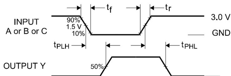
**Figure 1. Switching Waveforms**
