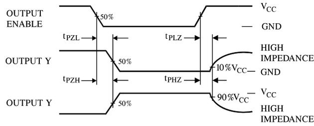
Figure 3. Switching Waveforms
