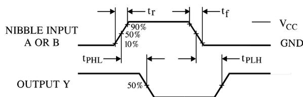
Figure 1. Switching Waveforms
