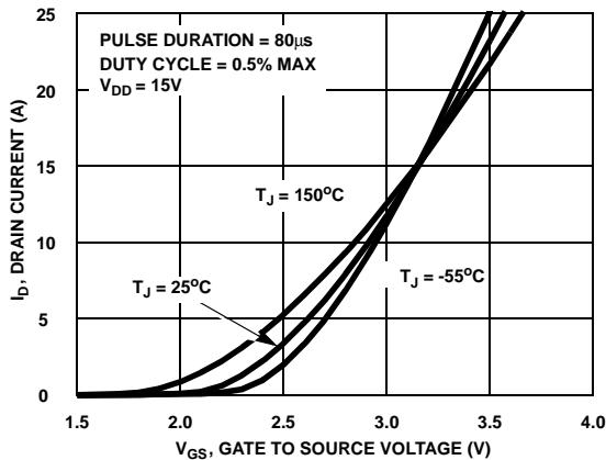
Figure 7. Transfer Characteristics
