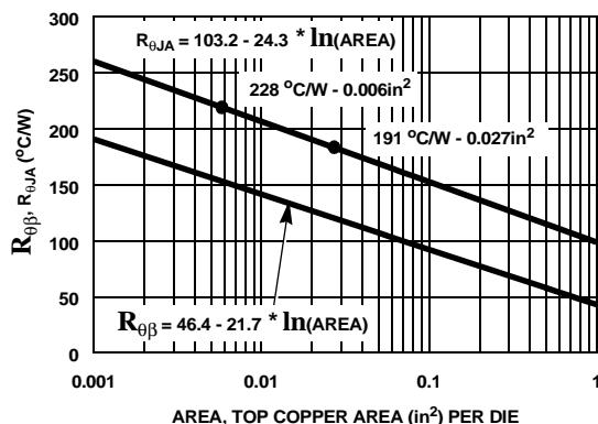
Figure 22. Thermal Resistance vs Mounting Pad Area
