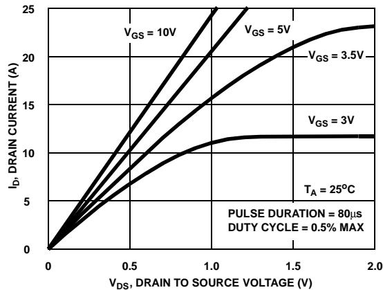
Figure 8. Saturation Characteristics
