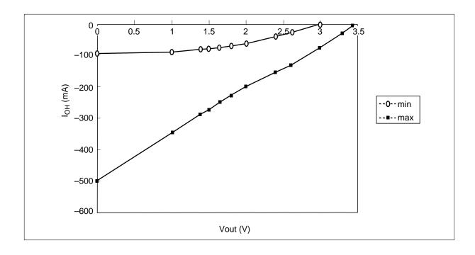
**DC Characteristics** (Ta = 0 to +70°C,  $V_{CC}$ ,  $V_{CC}Q = 3.3 \text{ V} \pm 0.3 \text{ V}$ ,  $V_{SS}$ ,  $V_{SS}Q = 0 \text{ V}$ ) (HM5225165B)
