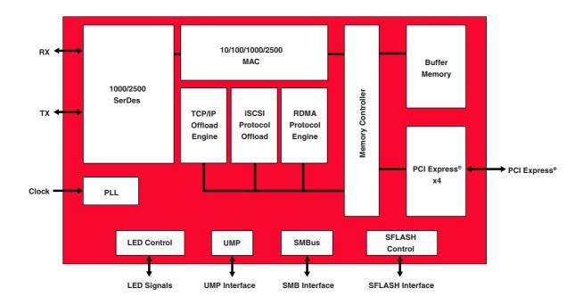
The BCM5708S provides a fully integrated Layer 4 and Layer 5 solution – TCP/IP, RDMA, and iSCSI along with a complete 1000/2500BASE-X Gigabit Ethernet, IEEE 802.3 compliant Media Access Control (MAC), and Physical Layer Transceiver solution for high performance network applications. By itself, the BCM5708S provides a complete single-chip Gigabit Ethernet NIC with a TCP/IP Offload Engine, RDMA NIC (RNIC), iSCSI HBA, or LOM solution.
